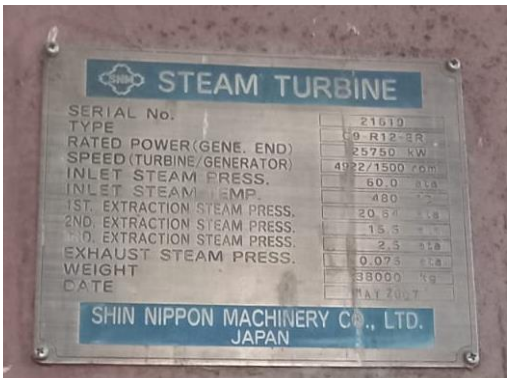
Figure 4: Nameplate details of the multi-stage steam turbine operating within the project discussed in this PCN.
